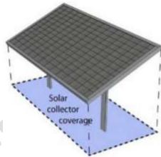
measured by the total surface area of the solar collector at maximum tilt to the vertical that occupies a given space or mounting surface, also referred to as the projected area of the array.
